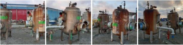
Manufacturer: Fluid Engineering Model: 723 Description: Motorized, automatic, selfcleaning strainers provide continuous debris removal from fluid piping systems that demand full time uninterrupted flow. Serial No: 7019 Year: 2012 Condition: Used Stock: 2
