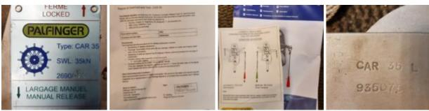
**Description:** The CAR 35 release hook meets the SOLAS standard for off-load release hooks and is dimensioned to suspend davit launched liferafts up to 40 persons and rescue boats with a davit load not exceeding 3.500kg. The red hand grip is designed for off-load release and the green hand grip is designed for on-load release.
