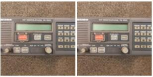
**Description:** All-in-one unit design including radiotelephone, DSC facility and watch keeping receiver Fully meets ITU, IEC, ETSI, IMO for GMDSS and other related standards Precision PLL frequency synthesizer for high frequency stability as required for DSC operation Output power 25 W, reducible to  $1~\rm W$
