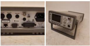
**Description:** The Agilent E4418B is a single-channel EPM series power meter, offering precise and reliable power measurements up to 26.5 GHz. This meter is widely used in RF and microwave testing environments, including research, manufacturing, and field applications.
