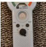
**Description:** The SKF TMEH 1 is a portable instrument that displays immediate information on the oil condition, which in many cases makes a lengthy laboratory investigation unnecessary. The unit
