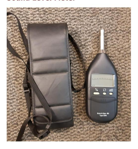
**Description:** Type 2240 is a very simple to use sound level meter, which complies with all the latest sound level meter standards. As an integrating-averaging sound level meter, it measures the equivalent, or average, sound pressure level Leq. In addition, it measures the instantaneous, maximum and peak sound pressure levels at the same time.
