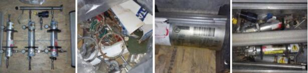
Manufacturer: Unknown Model: Unknown Description: Tightness test kit in hard case Kit with filter, three piston cylinders and spares Condition: Unknown Stock: 1
